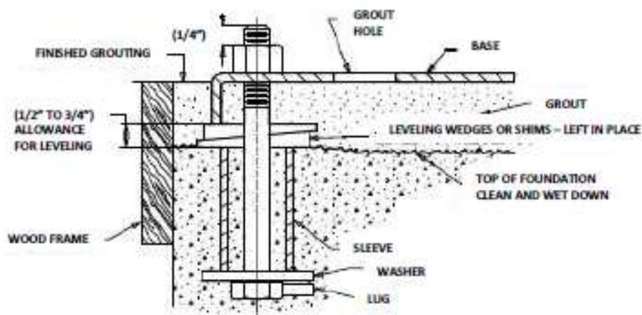
FIG. 3 TYPICAL FOUNDATION BOLT DESIGN
