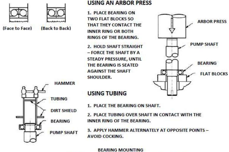
FIGURE 9 BEARING REMOVAL AND MOUNTING
