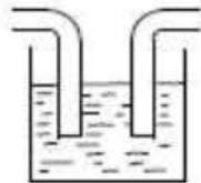
The supply line should extend down into the sump. Liquid supply entering a well perpendicular to the intake line tends to rotate the liquid, which interferes with the flow into the suction line (Figure 7).
