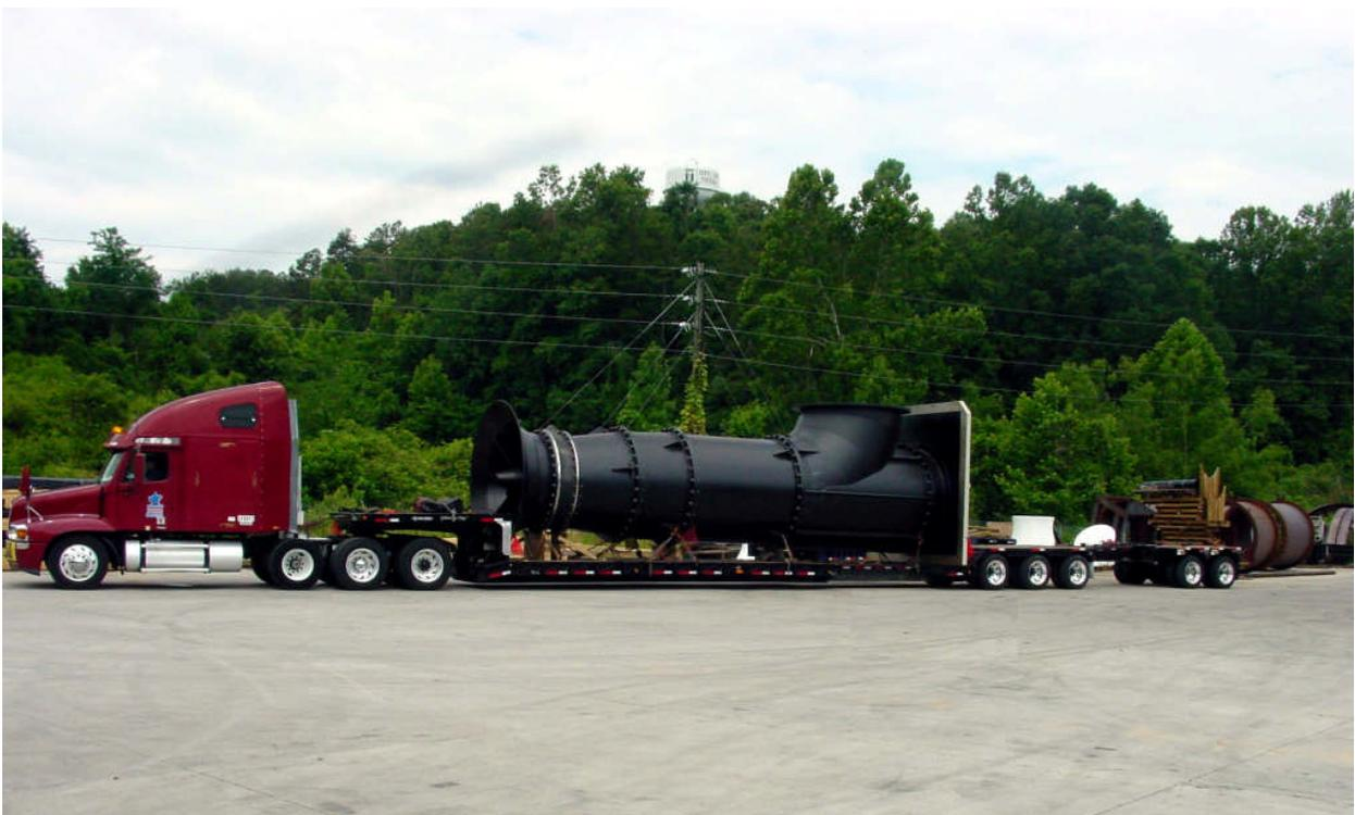
The massive Axial Flow Pump, which weighs approximately 110,000 lbs, has an 11-foot diameter suction bell and a 14.5-foot-square motor stand. It is driven by a 2,000 hp Caterpillar engine and moves water at the equivalent of seven average 35,000-gallon swimming pools every minute.
